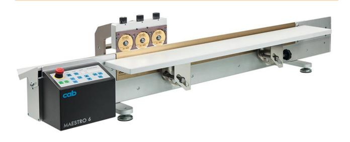
Cutting of pre-scored PCBs up to 1,500 mm length with minimum stress on components The MAESTRO 6 is the consequent further development of the proven cab depanelling machines.
