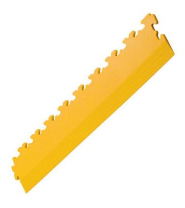
The 7mm thick X Joint ramp edge is designed to create a safe, sloped ramp onto your ESD floor tiles. Each ramp connects to a tile using the standard tap together interlocking joint. We recommend you use ramp edges in doorways and large entrances like shutters to eliminate trip hazards.
