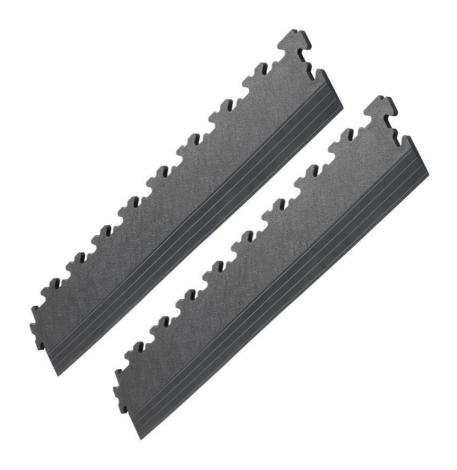
The 7mm thick X Joint ramp edge is designed to create a safe, sloped ramp onto your ESD floor tiles. Each ramp connects to a tile using the standard tap together interlocking joint. We recommend you use ramp edges in doorways and large entrances like shutters to eliminate trip hazards.
