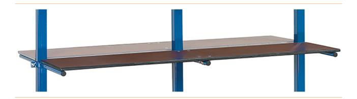
Accessories for standard support arm trolleys: wooden floor made of waterproof plywood 15 mm thick, can be used on both sides, one side is smooth, one side is anti-slip (silk-screen printed), with fastening clamps.
