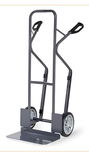
ESD tubular steel truck with sheet steel shovel, sturdy welded construction, electrically conductive powder coated, slate grey RAL 7015. ESD safety handles. Sheet steel shovel screwed on and therefore replaceable. Wheels with ESD solid rubber tyres, on plastic rims, hubs with roller bearings. Top bar and cross bars bent through. For the safe transport of round goods, such as rolls, cans, buckets, etc.
