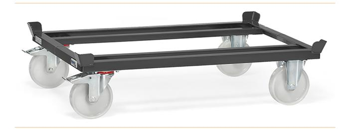
For flat pallets and mesh pallets. Robust welded angle steel construction, with 4 corners, powder coated, anthracite grey RAL 7016. 2 swivel and 2 fixed castors, polyamide wheels, hubs with roller bearings, brakes on swivel castors, in accordance with European standard EN 1757-3 (safety of platform trucks). Low rolling resistance, high chemical resistance, non-marking = non-marking. Driving noise.
