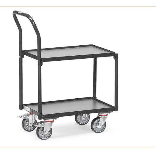
With 2 platforms and tubular push bar. Both frames with shelves made of derived timber material board, surface beech decor, edge 15 mm high. Powder coated anthracite grey RAL 7016. 400 mm clearance between shelves, total height 970 mm. Load capacity upper shelf 100 kg.
