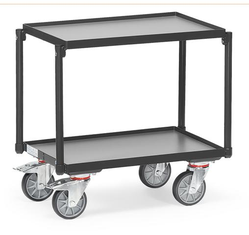
With 2 platforms. Both frames with shelves made of derived timber material board, surface beech decor, edge 15 mm high. Powder coated anthracite grey RAL 7016. 400 mm clearance between shelves, total height 639 mm. Load capacity upper shelf 100 kg.
