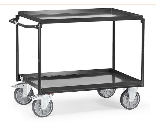
Welded steel construction. With 2 sheet steel trays. Tubular steel bracket and sheet steel trays screwed together. Trays oil-tight, rim 40 mm high. Powder coated RAL 7016 anthracite grey. Horizontal push handle. 2 swivel castors and 2 fixed castors, TPE tyres, hubs with deep groove ball bearings. Locks on swivel castors, in accordance with EN 1757-3 (safety of platform trucks). Load capacity upper platform 200 kg.
