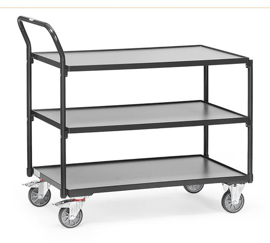
Light table trolley made of welded tubular steel and sectional steel, powder coated anthracite grey RAL 7016. Screw construction. 3 shelves made of derived timber material board, surface medium grey, lying in steel frame with 12 mm high edge. Push handle upright. 2 swivel castors and 2 fixed castors, TPE tyres, hubs with deep groove ball bearings. Locks on swivel castors, in accordance with European standard EN 1757-3 (safety of platform trucks). Load capacity upper and middle platform 80 kg.
