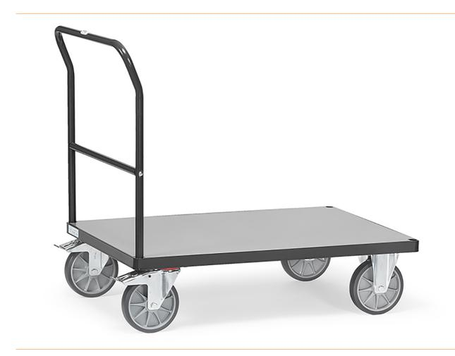
Pushbar trolley made of welded tubular steel and sectional steel, powder coated anthracite grey RAL 7016. Platform made of derived timber material board, surface medium grey. 2 swivel castors and 2 fixed castors, TPE tyres, hubs with deep groove ball bearings. Locks on swivel castors, in accordance with European standard EN 1757-3 (safety of platform trucks).
