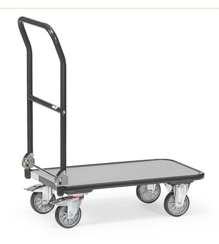
Folding trolley made of tubular steel, powder coated anthracite grey RAL 7016. Platform made of derived timber material board, surface medium grey. Folding push handle on platform. 2 swivel castors and 2 fixed castors, TPE tyres (non-marking), hubs with deep groove ball bearings. Locks on swivel castors, in accordance with European standard EN 1757-3 (safety of platform trolleys).
