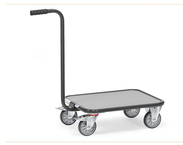
Handle roller in the "GREY EDITION" design. Made of welded tubular steel, powder coated anthracite grey RAL 7016. With wooden platform, platform with wooden material plate lying in the frame, surface medium grey. Handle can be screwed on. 2 swivel castors and 2 fixed castors, TPE tyres (non-marking), hubs with deep groove ball bearings, wheel stops on swivel castors, in accordance with European standard EN 1757-3 (safety of platform trucks).
