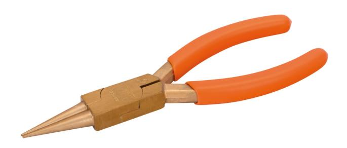
Non-sparking tools are used in areas where there is a potential fire and explosion hazard due to flying sparks. Round nose pliers made of copper beryllium, non-sparking,150 mm.
