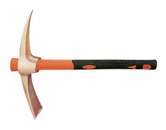
Non-sparking tools are used in areas where there is a potential fire and explosion hazard due to flying sparks. Non-sparking pickaxe made of copper beryllium, 385 mm x 910 mm.
