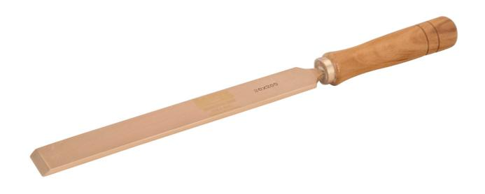
Non-sparking tools are used in areas where there is a potential fire and explosion hazard due to flying sparks. Flat scraper made of copper beryllium, non-sparking, 20 mm.
