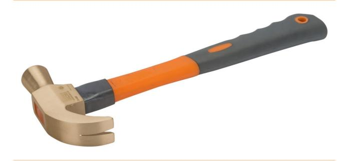
Non-sparking tools are used in areas where there is a potential fire and explosion hazard due to flying sparks. Claw hammer with copper beryllium head and fibreglass handle, non-sparking, 700 g.
