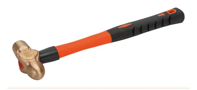
Non-sparking tools are used in areas where there is a potential fire and explosion hazard due to flying sparks. Engineer's hammer with ball tiller, copper beryllium head and fibreglass handle, non-sparking, 450 g.
