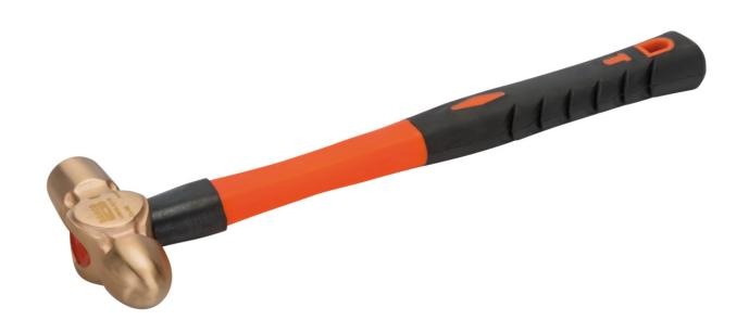
Non-sparking tools are used in areas where there is a potential fire and explosion hazard due to flying sparks. Engineer's hammer with ball tiller, copper beryllium head and fibreglass handle, non-sparking, 300 g.
