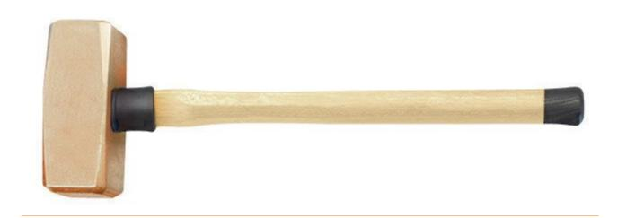
Non-sparking tools are used in areas where there is a potential fire and explosion hazard due to flying sparks. Mallet with copper beryllium head and wooden handle, non-sparking, 2.5 kg.
