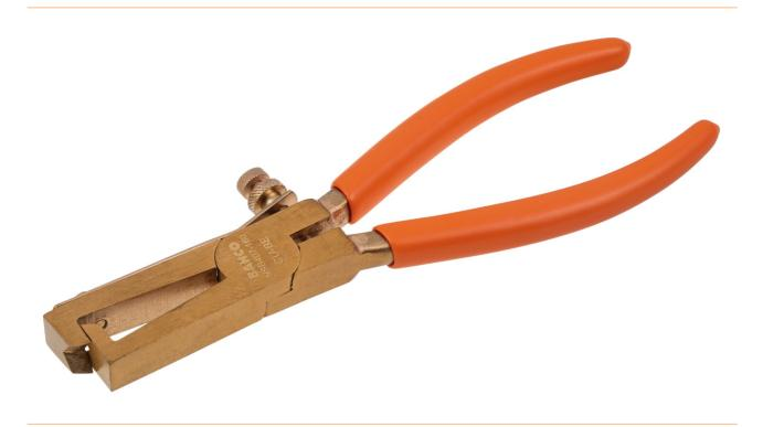
Non-sparking tools are used in areas where there is a potential fire and explosion hazard due to flying sparks. Stripping pliers made of copper beryllium, spark-free, 170 mm.
