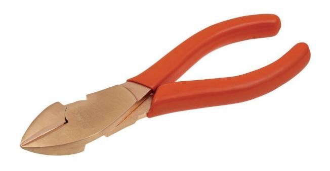
Non-sparking tools are used in areas where there is a potential fire and explosion hazard due to flying sparks. High performance side cutters made of copper beryllium, non-sparking, 160 mm.
