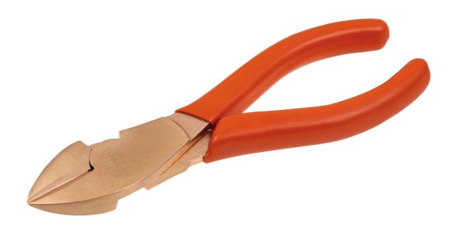
Non-sparking tools are used in areas where there is a potential fire and explosion hazard due to flying sparks. High performance side cutters made of copper beryllium, non-sparking, 160 mm.
