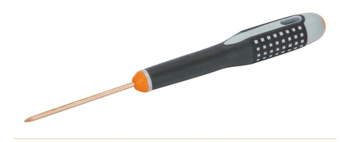
Non-sparking tools are used in areas where there is a potential fire and explosion hazard due to flying sparks. ERGO<sup>™</sup> Pozidriv screwdrivers made of copper beryllium, PZ2 x 125 .
