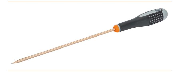
Non-sparking tools are used in areas where there is a potential fire and explosion hazard due to flying sparks. ERGO $^{\text{M}}$  Screwdrivers made of copper beryllium for slotted screws, electrician's blade, non-sparking, 0.5 x 3 x 50.
