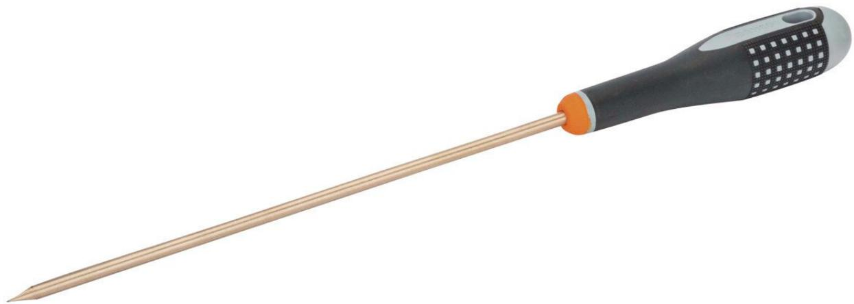
Non-sparking tools are used in areas where there is a potential fire and explosion hazard due to flying sparks. ERGO™ Screwdrivers made of copper beryllium for slotted screws, electrician's blade, non-sparking, 0.5 x 3 x 50 .
