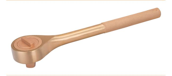
Non-sparking tools are used in areas where there is a potential fire and explosion hazard due to flying sparks. 3/4 reversible ratchet made of copper beryllium, non-sparking, 320 mm.
