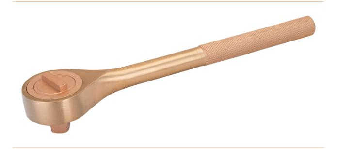
Non-sparking tools are used in areas where there is a potential fire and explosion hazard due to flying sparks. 1/2 reversible ratchet made of copper beryllium, non-sparking, 245 mm.
