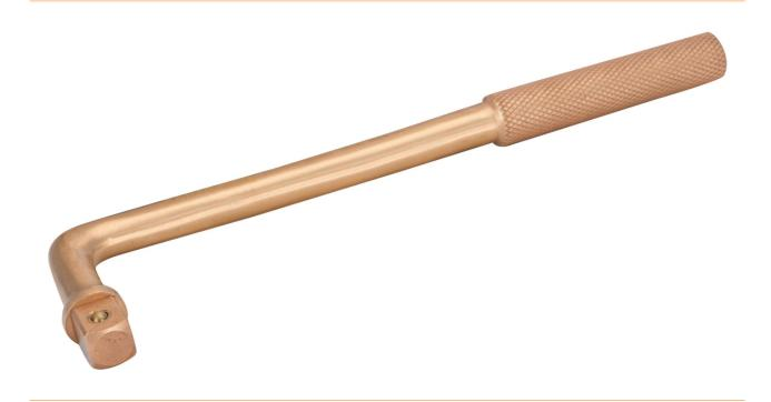
Non-sparking tools are used in areas where there is a potential fire and explosion hazard due to flying sparks. 1/2 angled copper beryllium handle, non-sparking, 230 mm.
