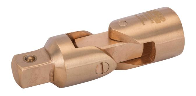
Non-sparking tools are used in areas where there is a potential fire and explosion hazard due to flying sparks. 3/4 drive cardan joint made of copper beryllium, 110 mm.
