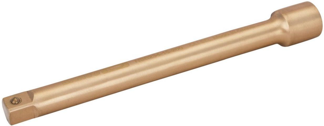
Non-sparking tools are used in areas where there is a potential fire and explosion hazard due to flying sparks. Non-sparking 3/4 extension in copper beryllium, 200 mm.
