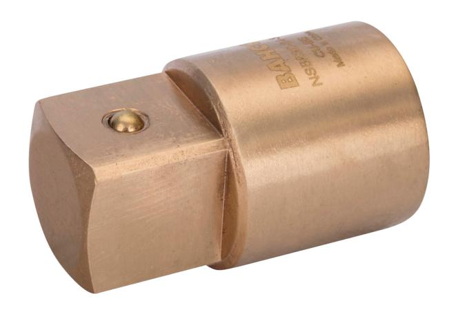
Non-sparking tools are used in areas where there is a potential fire and explosion hazard due to flying sparks. 1/2 to 3/4 adapter made of copper beryllium, with square drive.
