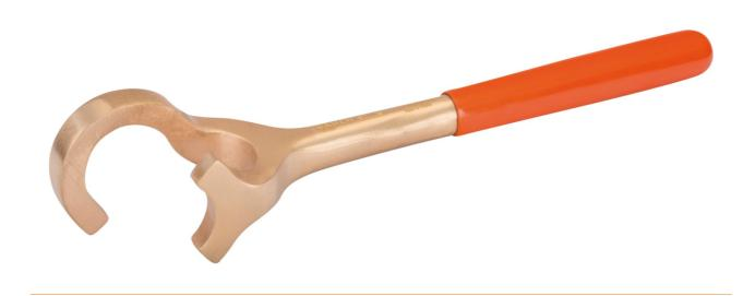
Non-sparking tools are used in areas where there is a potential fire and explosion hazard due to flying sparks. 32 mm valve wrench in copper beryllium, 215 mm.
