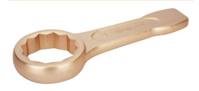
Non-sparking tools are used in areas where there is a potential fire and explosion hazard due to flying sparks. 89 mm striking-face box wrench made of copper beryllium, 380 mm.
