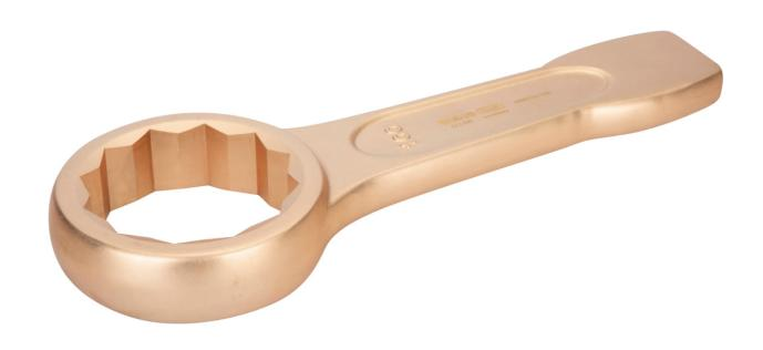
Non-sparking tools are used in areas where there is a potential fire and explosion hazard due to flying sparks. 88 mm striking-face box wrench made of copper beryllium, 380 mm.
