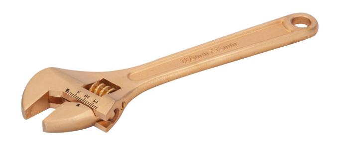
Non-sparking tools are used in areas where there is a potential fire and explosion hazard due to flying sparks. 36 mm copper beryllium wrench with central nut, 300 mm.
