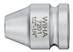
The connecting part with snap ring, external hexagon/external square, G 6.3 / G 10 / G 12.5 (01922), 35 mm from Wiha is ideal for use in automated screwdriving systems and manual applications. The output: DIN 3126, ISO 1173, shape D 6.3 + D 8 supports easy handling and reliable connections. Thanks to the robust design, the product is also suitable for intensive continuous use.
