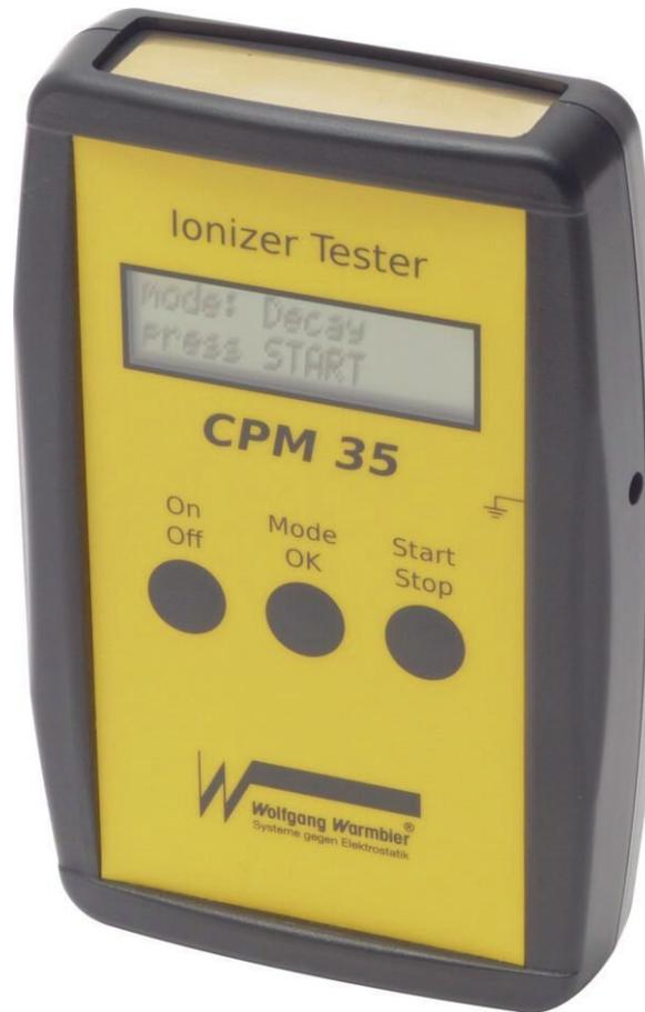
The CPM 35 is a handy measuring instrument for the fully automatic testing of ionizers at the ESD workplace or in machines. It measures positive and negative discharges as well as offset voltages and can also be used for periodic measurement of personal charges (walking test).
