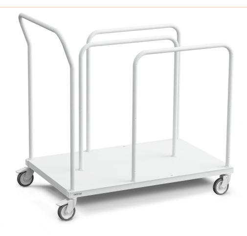
Trolley for large boxes. Three dividers can be mounted lengthwise or crosswise. The fourth divider acts as a push handle. Four swivel castors (Ø 100 mm), two of which have brakes. Height of the shelf above the floor 160 mm.
