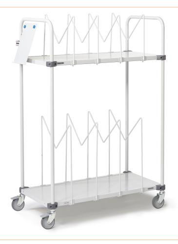
Trolley for packing cartons. Shelves with continuously adjustable M-divider brackets. Frame and individually height-adjustable shelves made of epoxy powder-coated steel. Height of the large divider brackets 540 mm, lowest point 330 mm above the lower shelf, height of the small divider brackets 315 mm, lowest point 105 mm above the upper shelf. Four swivel castors (Ø 100 mm), two of which have brakes.
