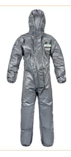
Polymer-coated chemical protection suit, hood with face rubber, tight mask closure, elasticated arm and leg ends, hot-taped seams, adhesive double zipper cover, impressive softness and suppleness, low-noise material, padded double-layer knee pads, barrier against a wide range of chemicals, heat-sealed seams. against a wide range of chemical warfare agents and aggressive chemicals as well as biological hazardous substances, antistatic on the inside
