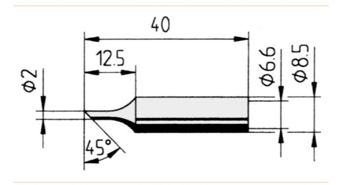
• Continuous soldering tip, straight, bevelled 45° angle, 2.0 mm diameter, with ERSADUR-LF coating (lead-free soldering) for increased service life.
