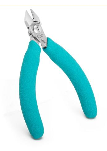
The jaws of the cutter have straight edges and taper to a point. This head shape allows access to difficult to reach areas but reduces the cutting capacity in comparison to the same size oval head cutter.
