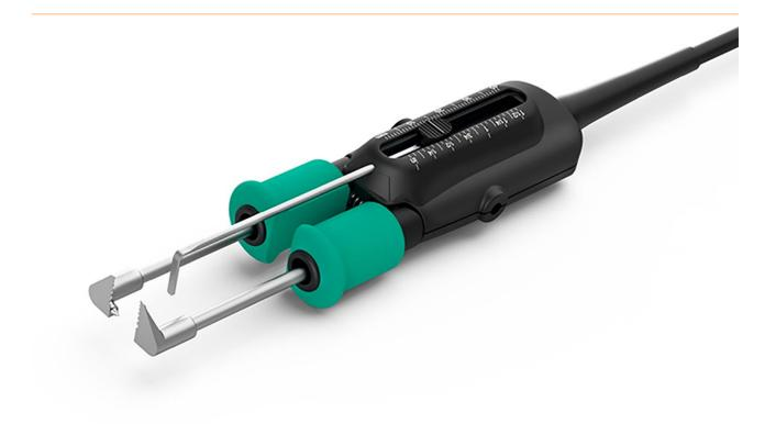
The WS440 is specially designed for stripping high temperature cables made of thermostable materials such as Teflon\*, Kapton\*, silicone rubber, etc. from 34 to 16 AWG (0.16 to 1.29 mm) at temperatures up to 800  $^{\circ}$ C / 1470  $^{\circ}$ F.
