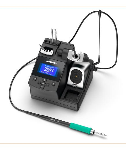
The JBC CD-2BQF is a Compact Series digital soldering station designed specifically for general electronics applications. With an output of 130 W, it offers precise temperature control and is therefore ideal for processing SMD and THT components. The station is supplied with the T245-A soldering handle, which is compatible with a wide range of C245 soldering tips. Optionally, the T210-A and T210-PA handles can also be used, further increasing the versatility of the station.
