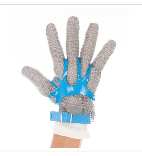
Sting protection gloves without cuff from Hygostar: The sting protection glove is made of a mesh of stainless steel rings, which have a diameter of 4mm. The glove does not have a cuff, but can be adjusted to fit perfectly by the proven push-button technology. In addition, a quick removal of the glove is possible. The stab protection glove is suitable for both left and right handers. The possibility of easy and residue-free cleaning of the glove makes it ideal for the food industry.
