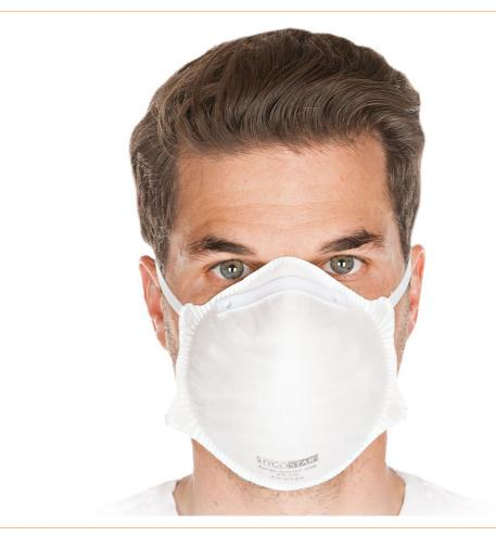
The FFP2 NR respirator is made of white polypropylene. This mask has two head straps, a flexible noseband and a soft nosepad, which ensures a good fit and high wearing comfort. In addition, the FFP2 NR respirator is very durable. This mask is an ergonomic fine dust mask that provides good protection against hazardous dry particles and aerosols (e.g. metal dusts, mineral fibre dust, polishing dusts, construction site dusts).
