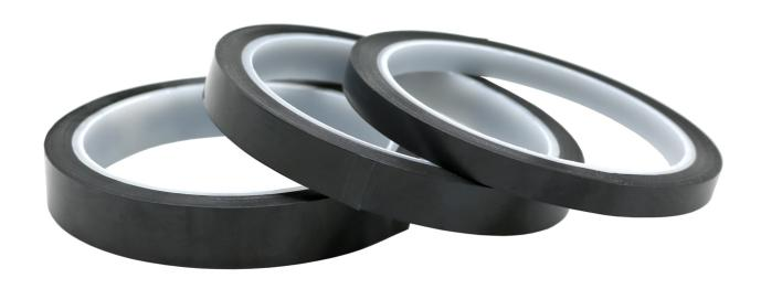
The ESD Kapton adhesive tape from Safeguard in the color black reliably protects against damage caused by electrostatic discharge to electronic devices and components. The Kapton adhesive tape with a width of 6 millimeters and a length of 33 meters made of polyimide has an excellent heat and chemical resistance. It is widely used in the electronics industry due to its very good insulation and high temperature resistance.
