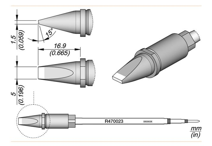
Special tips for use in automated soldering processes
