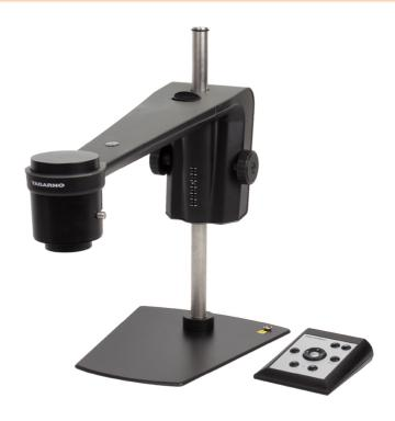
The Tagarno TREND automated digital microscope and inspection system in black includes the XPLUS control box, 4x zoom (4+) objective, watermark, focus stack and ruler in this set. The Tagarno Trend is an agile and personal digital microscope that fully adapts to the needs of the user. It impresses with 30x optical zoom, 60 FPS frame rates, 385 mm working depth, 1080p image quality as well as up to 330x magnification.
