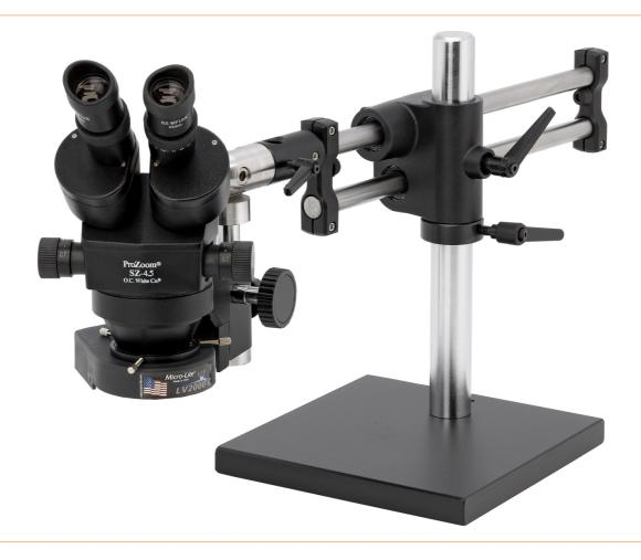
The ProZoom® 4.5 ESD stereo microscope from O.C. White excels as an inspection instrument with extended working distance and exclusive, taut zoom stops, as well as an extra-large (22mm) 10X eyepiece standard range 7-45X (3.5 - 225X with optional parts).
