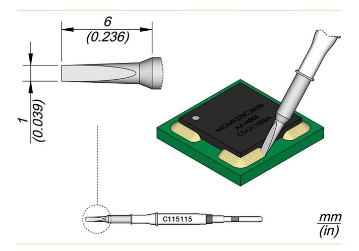
The C115 series soldering tips are suitable for soldering and repairing very small components. These are compatible with NT115-A, NP115-A and AN115-A Nano soldering handpieces.
